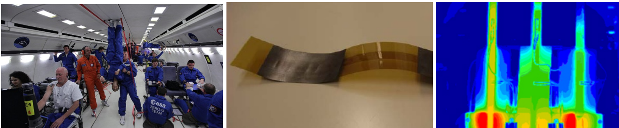
Experiments on flexible heat pipes during parabolic flights of the European Space Agency (ESA)
